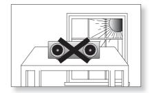
Do not expose the unit to direct sunlight or other heat sources. This could cause the unit to overheat and malfunction.
